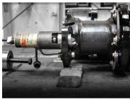
Replacing of spherical bearings
